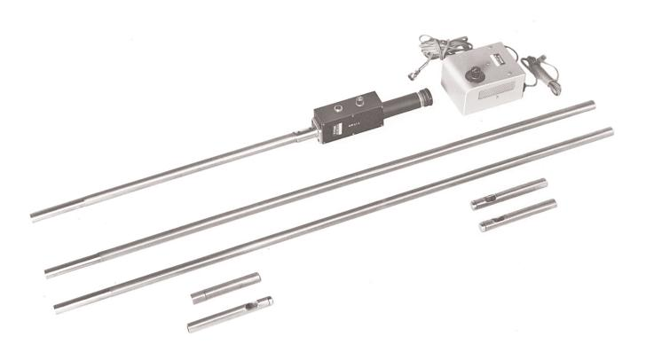
D Series borescopes are designed for extended-length viewing and general use in inspection areas of 0.803" (20.4mm) or larger. The basic model has a working length of 22" (558.8mm) and includes two 40" (1016mm) sections to extend working lengths to 62" (1574.8mm) and 102" (2590.8mm). Additional 40" extensions are available - up to six extension pieces are recommended for use to 240" (6096mm) working lengths.
